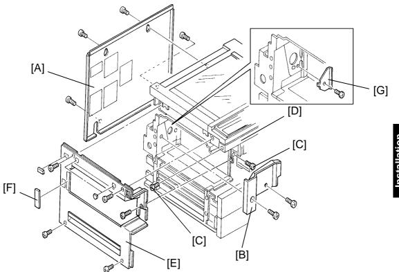
**NOTE:** The sorter adapter is required to transport copy papers from the copier exit rollers to the sorter entrance guide plates. It is required when the mini-sorter (A423), midi-sorter (A411), or sorter stapler (A366) is installed.
